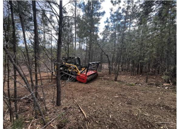
Masticator implementing fuels reduction work during project implementation in 2024.
